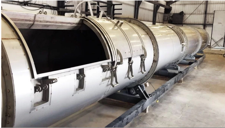
In-Vessel Composting System
