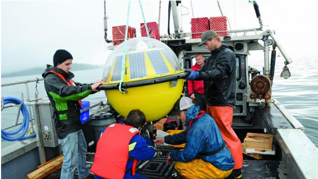
*Wave-measuring buoys like this one were used in a new study to measure wave energy potential off the coast of Vancouver Island | Submitted*
