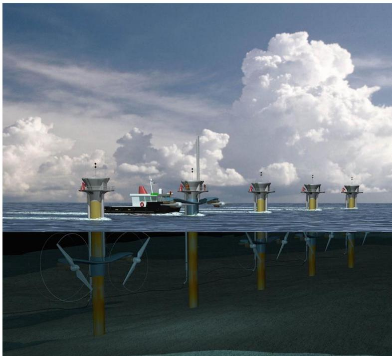
*Tidal turbines harness marine currents and tidal energy using tidal stream turbines that work much like submerged windmills, but are driven by flowing water rather than by air. Marine Current Turbines*
