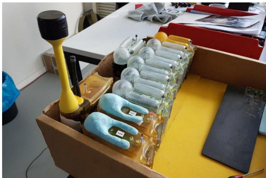
Funded through a grant from Switzerland’s [Nano-Tera](#) program, Envirobot comprises several modules. Some of these contain conductivity and temperature sensors; others have miniaturized biological sensors that harbor bacteria, small crustacean, or fish cells that respond to water toxicity in different ways.
