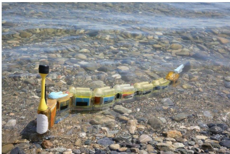
Even for an automaton, Envirobot is uncommonly clever. Besides its capacity to follow a preprogrammed path, it can also make its own decisions, independently sniffing out the origin of the contamination.
