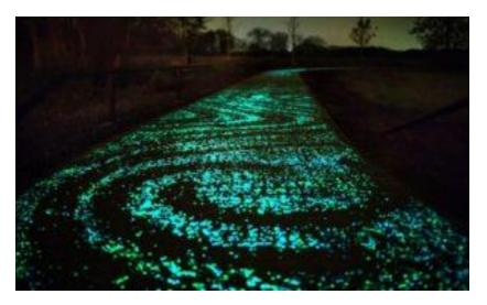
Glowing Bike Path The cement is designed to take in solar energy, which can be emitted at night as light.
