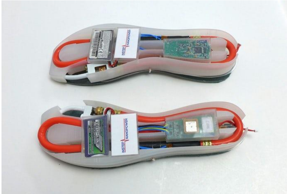
The researchers combined reverse electrowetting with a novel device called a bubbler. UW-Madison College Of Engineering
