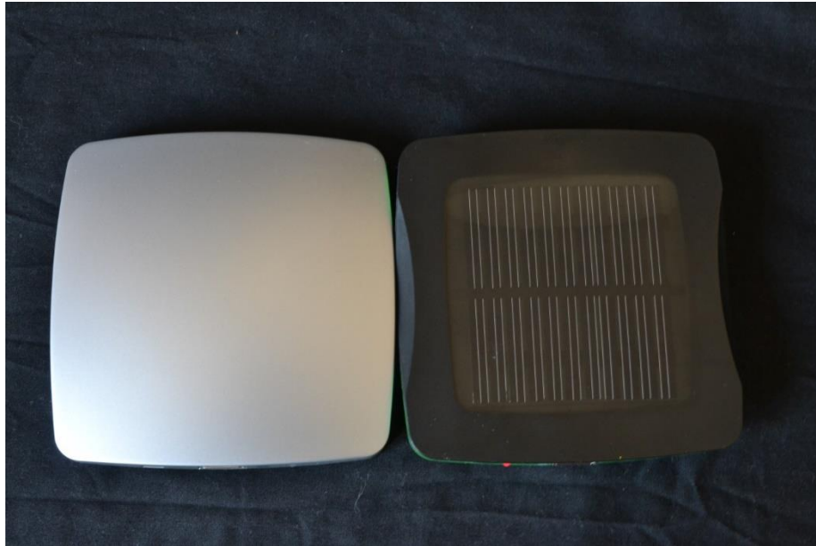
The Window charger features a 110 mA rated 7.8 x 7.8 mm PV panel
