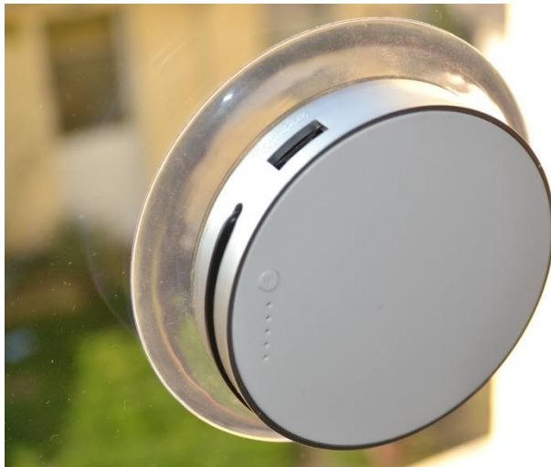
When charging by bright (sun)light, the green LED will light up
