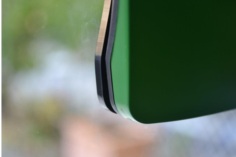
The curve to the PV face caused the charger to pull away from the supplied silicone ring, and fall
