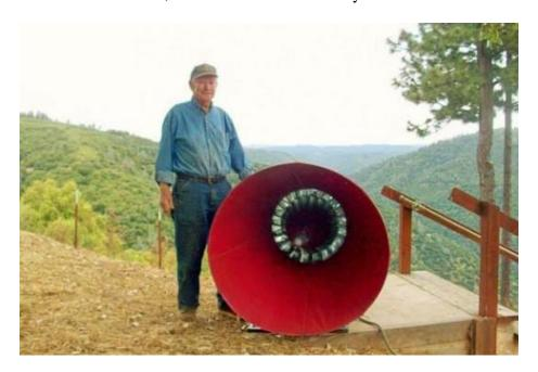
The CWP turbine uses their patented Inner Compression Cone Technology, which is claimed to squeeze and compress the incoming air in order to be able to create more power at the turbine.
