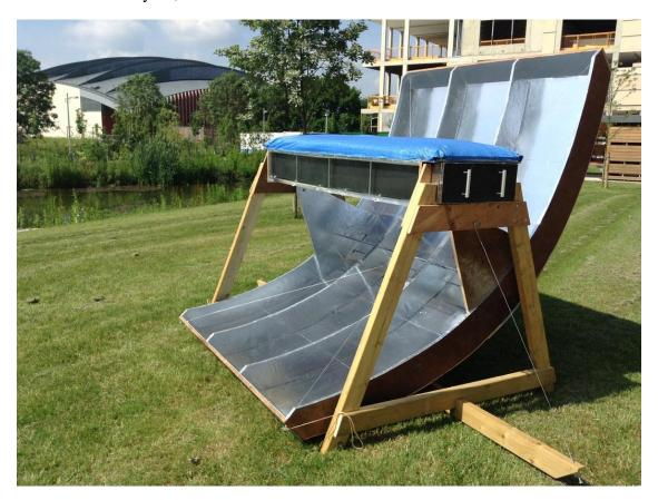
The Infinity Oven is a low cost solution which enables bakery entrepreneurs and communities in the developing world to harness the power of the sun, baking and cooking more sustainably: smoke free and fuel free.
