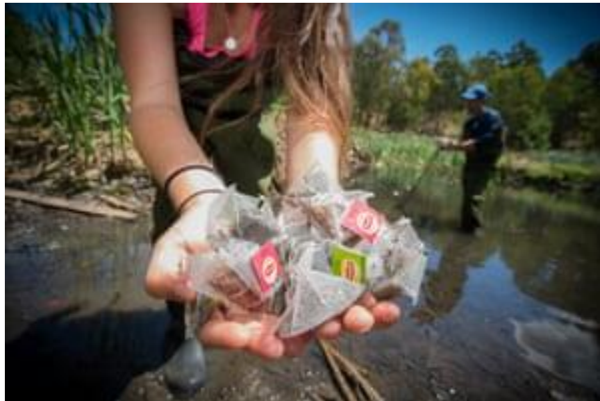
Lipton teabags are being used in the research as they have a fairly standard rate of decay in wetlands. Photograph: Simon Peter Fox
