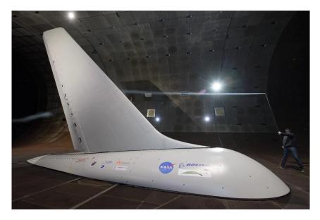
Researchers with NASA's Environmentally Responsible Aviation project coordinated wind-tunnel tests of an Active Flow Control system -- tiny jets installed on a full-size aircraft vertical tail that blow air -- to prove they would provide enough side force and stability that it might someday be possible to design smaller vertical tails that would reduce drag and save fuel. Credits: NASA/Dominic Hart
