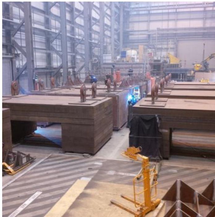
Atlantis Resources. Each ballast block, which anchors the tripod of the turbine, weighs 200 tonnes.
