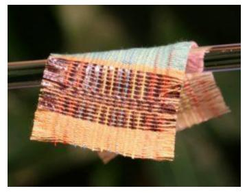
A piece of fabric woven with special strands of material that harvest electricity from the sun and motion.
