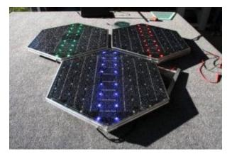
Solar Roadways's hexagonal solar panels feature LED lighting and smart technology that allows them to "communicate" with each other. Photo credit: Solar Roadways
