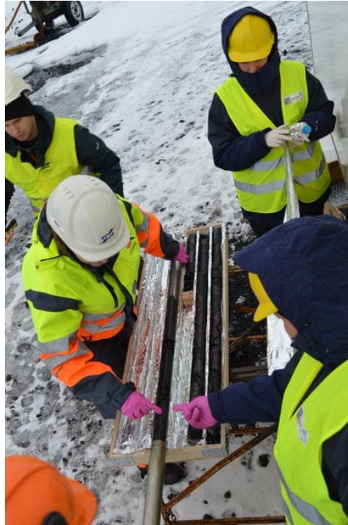
Members of the CarbFix science team handling rock core recovered during drilling at the CO2 injection site. Photograph: Juerg Matter/Science
