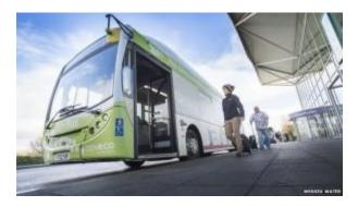
The 40-seat "Bio-Bus" runs on biomethane gas generated through the treatment of sewage and food waste.
