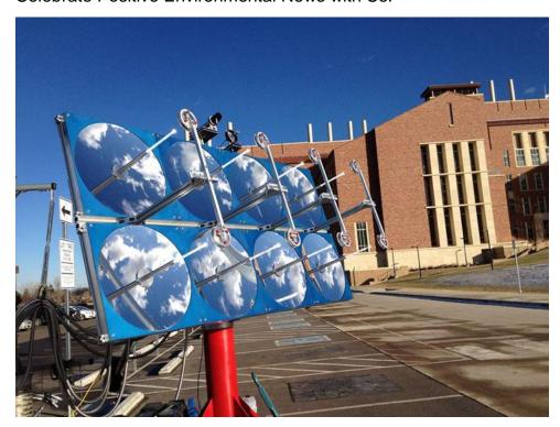
The Sol-Char toilet is outfitted with <u>eight parabolic mirrors</u> that reflect the sun's rays and divert it to a postage stamp-sized point. Up to 700 watts of solar energy collected at this point is then directed to cables in the reaction chamber system, which helps to burn the poop inside with temperatures reaching a whopping 600 degrees Fahrenheit. The burned-up poop then has a charcoal-like quality, making it easy to transport, distribute, and use in soil.
