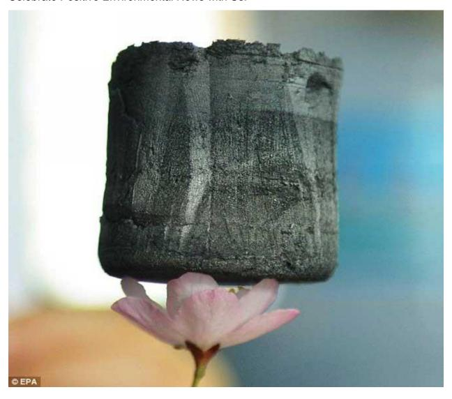
The lightest solid ever developed: A piece of graphene aerogel developed in a lab at Zhejiang University is placed on a cherry flower in Hangzhou in east China's Zhejiang province
