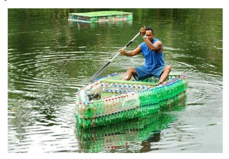
600 littered plastic bottles were used by Tom Davies, a New Zealand native living in Fiji, to create this boat. It measures 4.5 metres long and 1.4 metres wide. All the 600ml bottles used are glued together to a layer of foam underneath. In Tom's tests, the boat can hold up to three big Fijian men.
